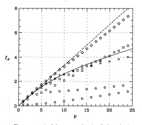
Figure 4: The exponent  $\zeta_p$  of the structure function  $S_p$  shown by  $\diamond$ ,  $\Box$  and  $\odot$  which are as in figure 3. dashed line, K41 (1.13); solid line, log-Poisson model (1.17);  $\times$ , DNS at  $R_{\lambda} = 150$ , Vincent & Meneguzzi (1991) [1]; +, jet at  $R_{\lambda} = 852$ , Anselmet *et al.* (1984) [11].
