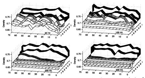
Figure 10: Density response for non-spherical glass beads with an an average density of 0.68. .
