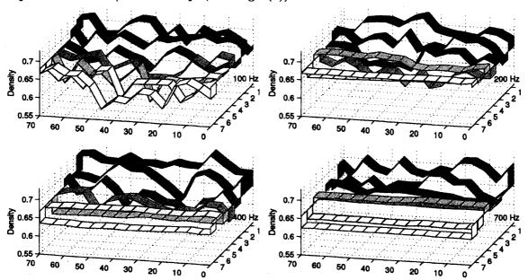
Figure 7: Density response for spherical glass beads with an an average density of  $\rho = 0.66$ , for all seven sensors (x-axis) between 0 and 70 seconds (z-axis).
