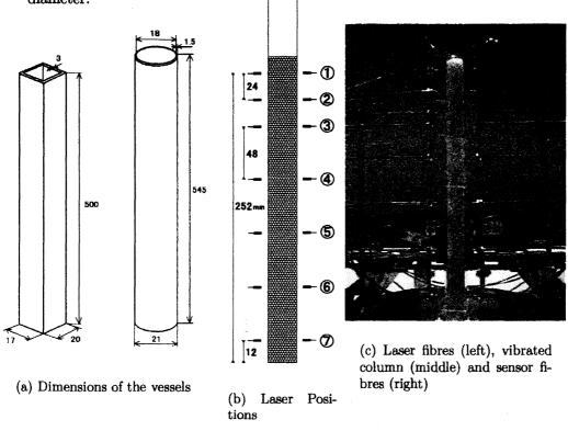
Figure 1: Dimensions of the setup
