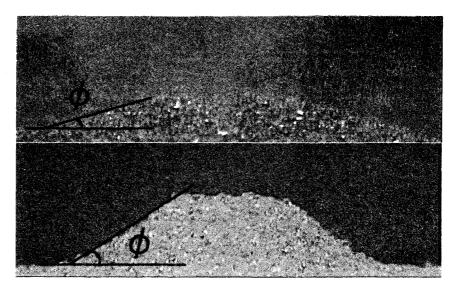
(b) Critical angle for the spherical beads  $(17^o,above)$  and non-spherical beads  $(32^o,below)$
