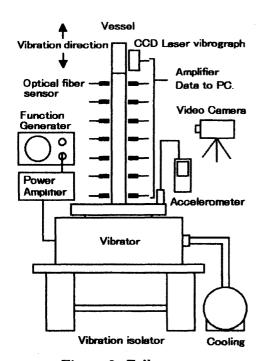
Figure 2: Full setup the effect of subtle changes in the setup.
