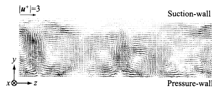
Fig.24 Time-averaged velocity distribution on z - y section
