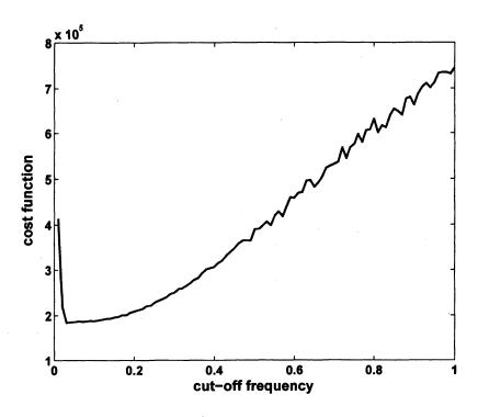
🗵 5 The cut-off frequency dependence of the cost function
