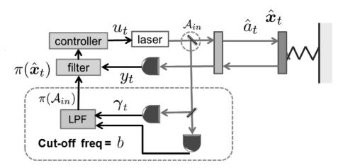
🗵 3 Schematic of the adaptive quantum Kalman filter and LQG controller.
