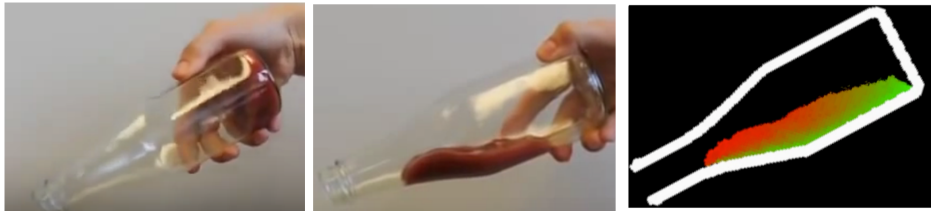
FIGURE 1: Hydrophilic vs. hydrophobic surfaces: no-slip vs. slip condition. Left: Classical Ketchup flow. Middle: Ketchup flowing in a bottle treated with a no-stick coating. Right: Our numerical simulation of flow with slip boundary condition. The pictures were taken at the same moment in time after the bottle throat started pointing downward.
