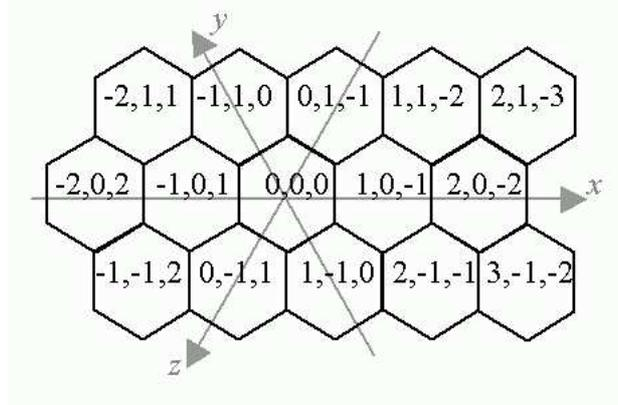
FIGURE 4. Coordinate values on the hexagonal grid
