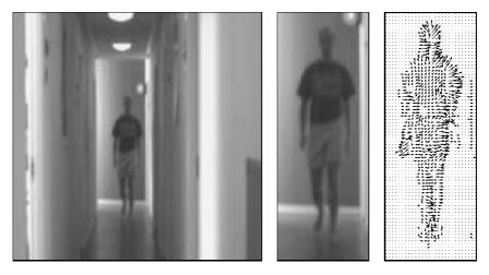
Figure 3. (a) Left: One frame of a hallway sequence with  $256 \times 256 \times 16$  pixels. A person is approaching the camera. (b) MIDDLE: Detail. (c) RIGHT: Computed optic flow. From [38].
