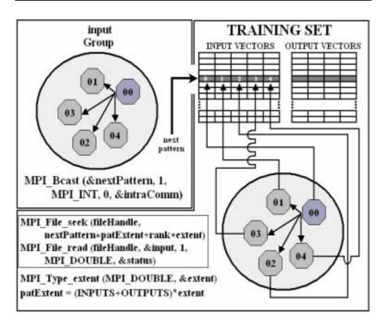
Figure 5: The retrieval of the training pattern input values from the processes of the input group
