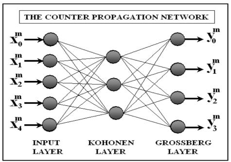
Figure 1: A typical counter - propagation network
