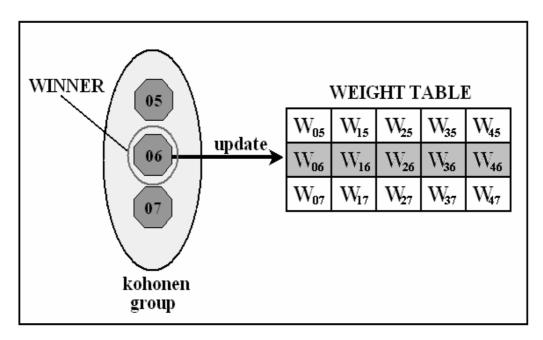
Figure 7: The update of the synaptic weights associated with the winning process
