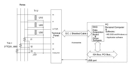
Figure 1. Basis scheme the of the quality analyzer
