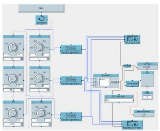
Figure 2. The simulator program for homopolar components
