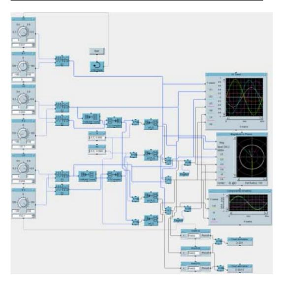
Fig.6. The graphical program for simulation symmetrical components
