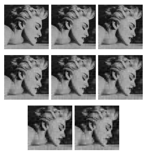
Below are the results of the picture where all wavelet coefficients smaller than 1 percent of the largest are deleted when the wavelet used is  $D_4$ ,  $D_{12}$  and  $D_{20}$  respectively. The compression factors are 135, 146 and 145 respectively. Note that for  $D_{20}$  the picture is smoother than for  $D_4$ . This smoother situation is closer to what would be obtained by a Discrete Fourier Transform.
