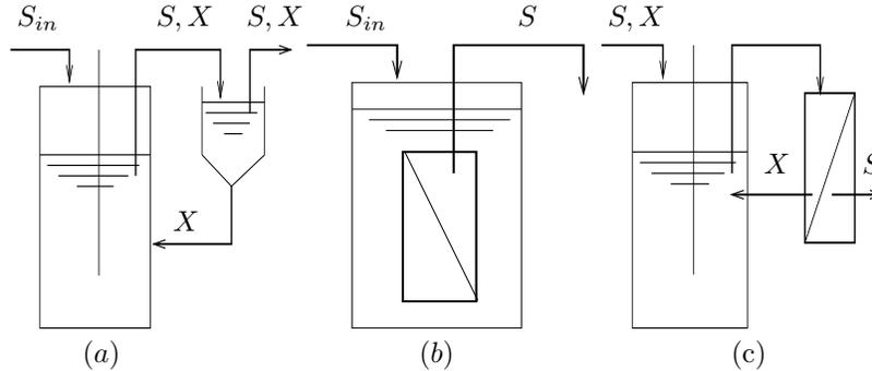
FIGURE 1. Membrane Bio-Reactor : (a) Conventional activated sludge process, (b) Submerged MBR configuration with integrated membrane unit, (c) Side stream MBR configuration with external membrane unit.
