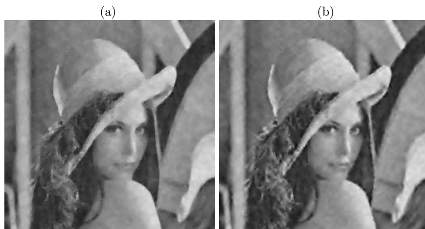
FIGURE 3. Lenna: Restored images (best in PSNR) by (a) the ITV model and (b) a fourth-order model, that shows PSNR=26.88 (SNR=131.51, CPU time=0.28 seconds) and PSNR=27.44 (SNR=149.63, CPU time=42.88 seconds), respectively.
