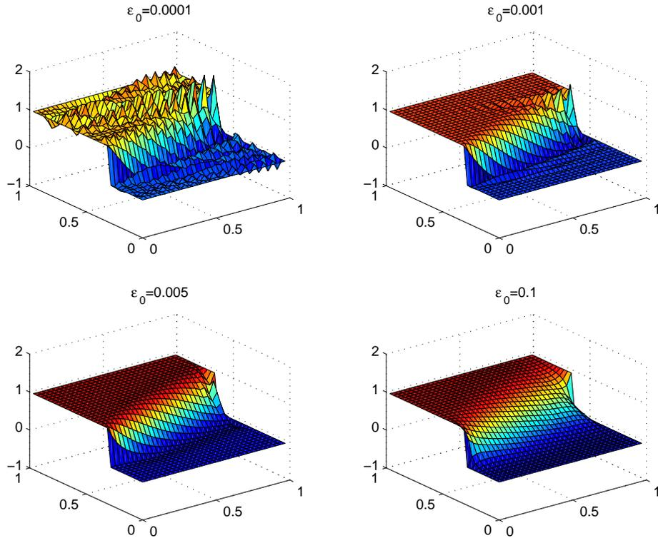
FIG. 4.1. Spatial stability of the steady-state solution for various choices of the artificial viscosity parameter  $\epsilon_0$ .
