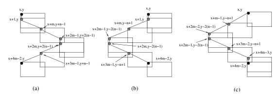
FIG. 3.8. Two transformations to replace vertical edges in  $G_s$ . (a) The regular vertical edge transformation, (b) its mirror image and (c) version only used for an upward edge of a T-junction. Dark nodes are for original vertices, and shaded nodes correspond to auxiliary vertices to replace an edge between them. Dark edges correspond to edges in  $G_L$ , and rectangles are also drawn to illustrate overlaps.
