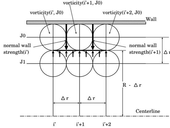
FIG. 4.2. Balance of NWS and pressure at wall.
