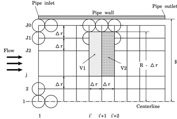
FIG. 4.1. Grid system,  $\Delta x = \Delta r$ .
