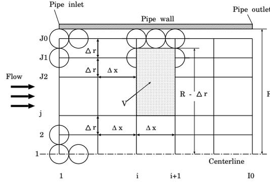
FIG. 2.1. Grid system in a circular straight pipe.
