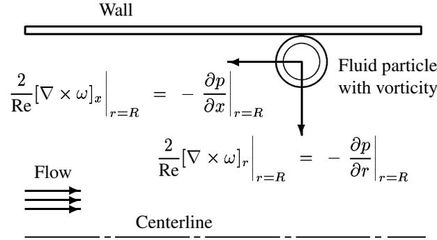
FIG. 3.1. Directions of curl of vorticity at wall.
