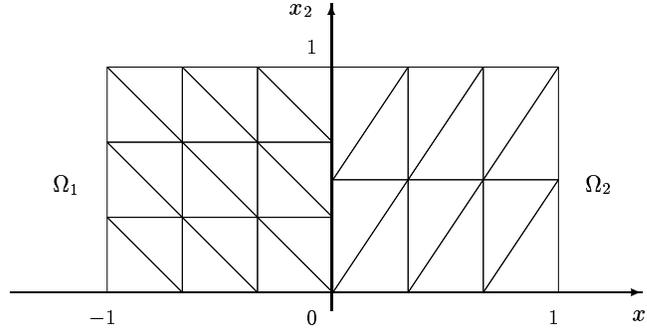
FIG. 6.1. Initial triangulation (first example).
