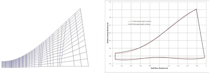
FIG. 4.2. Initial steam path contour (left panel), and Initial and optimized steam path contours (right panel).
