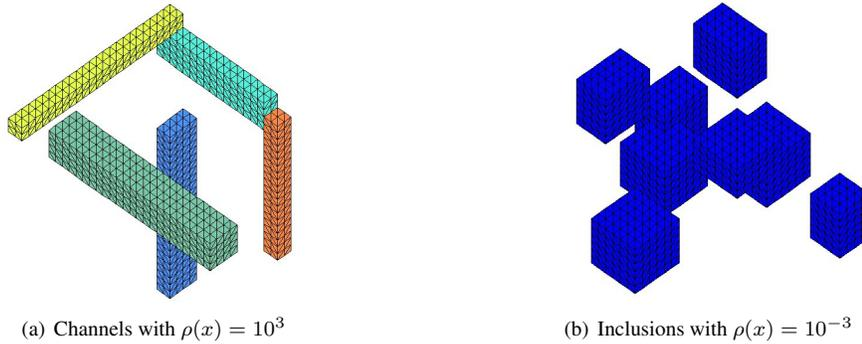
FIG. 6.3. Coefficient distribution with channels and inclusions: channels ( $\rho(x) = 10^3$ ), small cubes ( $\rho(x) = 10^{-3}$ ), and elsewhere ( $\rho(x) = 1$ ).
