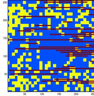
FIG. 6.1.  $\rho(x)$  with channels and inclusions: channel ( $\rho(x) = 10^3$ ), inclusion ( $\rho(x) = 10^{-3}$ ), and elsewhere ( $\rho(x) = 1$ ).
