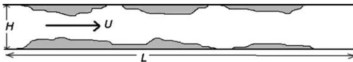
Figure 1. Flow in a long thin channel with aspect ratio \varepsilon := H/L \lll 1 : The biofilm growing on the walls of the channel (grey region \Omega_2(t) ) induces a perturbation of the Poiseuille profile that is observed in an empty flow channel. In the white region \Omega_1(t) the flow field is described by the flow model (6).
