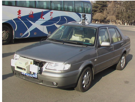
Figure 1: Multisensor based pedestrian recognition experimental platform.
