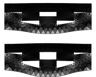
FIGURE 6.14. Tresca criteria for the stresses in the viscoelastic (0.5, 0.2) and elastic cases.
