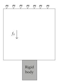
FIGURE 4.5. Contact problem of a 2D viscoplastic body.
