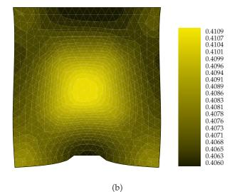
$\ensuremath{\mathsf{Figure}}\xspace 4.7.$  Von Mises stress norm and damage field at final time in the deformed configuration.
