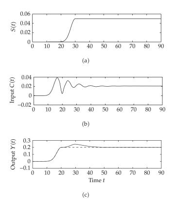
FIGURE 5.1 Closed loop simulation: (a) the input substrate concentration S, (b) the feedback control C, and (c) the reference output  $Y^*$  (dotted) and the resulting output Y (solid).
