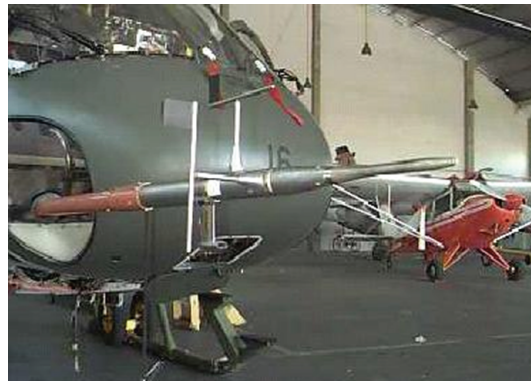
Figure 2: "Squirrel" AS355-F2 helicopter and installed nose boom.
