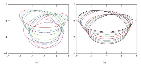
**Figure 6:** Transformation of the trajectory of the vector rotator  $\overrightarrow{\Re}_{022}$  (and  $\overrightarrow{\Re}_2$ ) in the plane through pole  $O_2$  and orthogonal to the self rotation axis for different values of parameter  $\psi$ .
