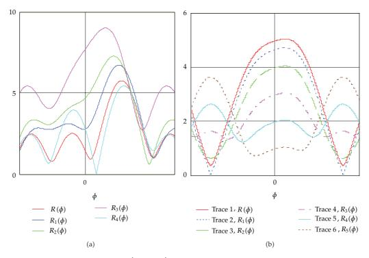
Figure 5: Intensity of vector rotators  $\overrightarrow{\mathfrak{R}}_{022}$  and  $\overrightarrow{\mathfrak{R}}_{2}$ , for different disk eccentricity (a) and for different initial conditions (b).
