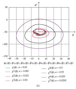
**Figure 7:** Transformation of the trajectory of the vector rotator  $\overrightarrow{\mathfrak{R}}_{022}$  (and  $\overrightarrow{\mathfrak{R}}_2$ ) in the plane through pole  $O_2$  and orthogonal to the self rotation axis, for different values of parameter a, orthogonal distance between axes of gyrorotor-disk coupled component rotations.
