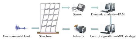
Figure 1: Schematic diagram of MBC nonlinear control strategy based on FAM.
