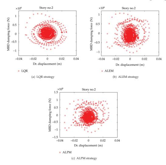
Figure 9: MRD damping force versus storey displacement under El Centro seismic excitation.
