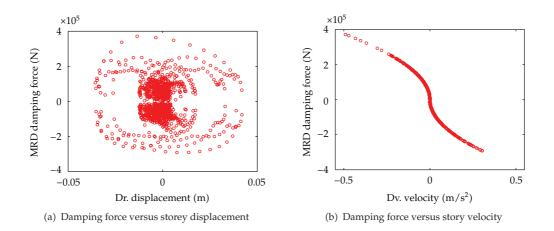
Figure 5: MRD damping force versus storey displacement and storey velocity under El Centro seismic excitation.
