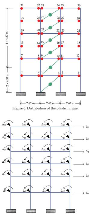
Figure 7: Numeration of structural degree of freedom.
