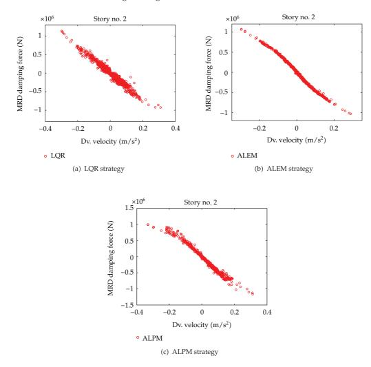
Figure 10: MRD damping force versus storey velocity under El Centro seismic excitation.
