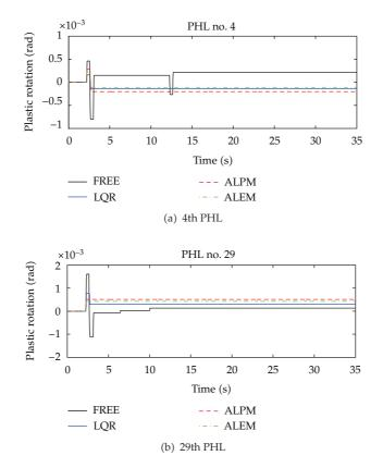
Figure 8: Rotations curves versus time history of the 4th and 29th PHL under El Centro seismic excitation.
