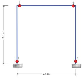
Figure 2: The sketch and PHLs of the structure.
