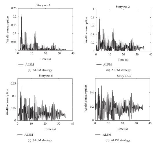
Figure 12: Wealth consumption curves versus time history of second floor and top floor under El Centro seismic excitation.
