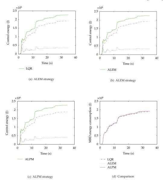
**Figure 13:** Structural energy response with LQR and MBC strategy under El Centro seismic excitation. Solid green line: IE, dashed pink line: CE, dotted black line: KE+DE+SE.
