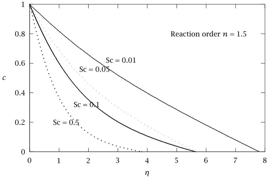
FIGURE 5.8. Concentration profiles for  $n = 1.5$ .
