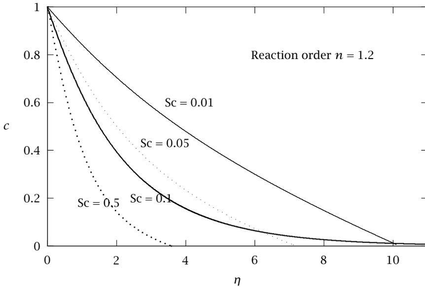
FIGURE 5.6. Concentration profiles for  $n = 1.2$ .
