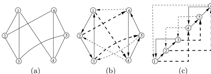
Figure 13: (a) A graph  $G = (V, E)$  of degree three. (b) The regular directed multigraph  $G' = (V, E')$  with indegree and outdegree equal to two obtained from  $G$  and its directed 2-factors  $C_1$  and  $C_2$ . The edges of  $C_1$  are represented by solid lines and the ones of  $C_2$  by dashed lines. Edges not in  $G$  are thinner than the other edges. (c) The RAC drawing of  $G'$  with one bend per edge constructed by the algorithm described in the proof of Theorem 7.
