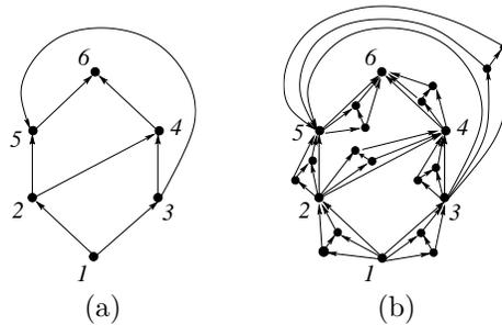
Figure 7: (a) A planar acyclic digraph  $G$  that is not upward planar. (b) The planar acyclic digraph  $G'$  obtained by replacing each edge of  $G$  with a copy of  $H$  is not straight-line upward RAC drawable.
