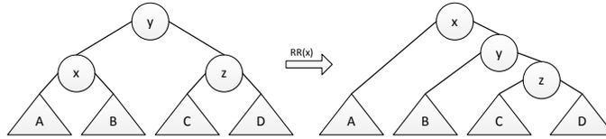
Figure 1: A single right rotation of node  $x$ . The triangles represent (possibly empty) subtrees that are not changed by the rotation.
