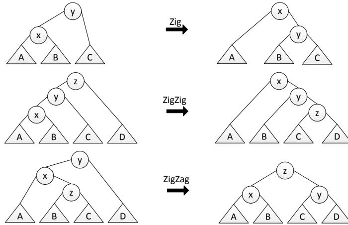
Figure 11: The three basic splay operations of splay trees.
