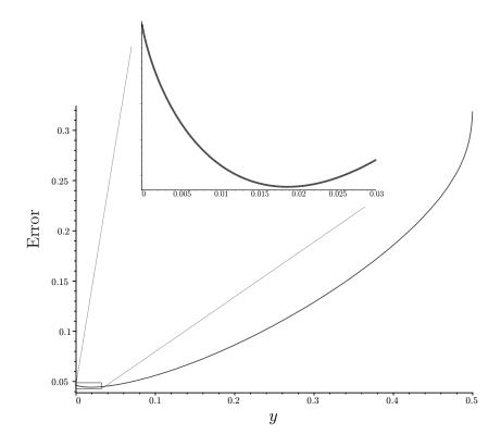
Figure 3.2: Numerical error,  $|f(a) - f^*(a)|$ , as a function of collocation point y. The zoomed graph indicates an optimal collocation point near y = 0.019
