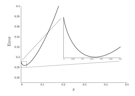
Figure 3.1: Theoretical error given by equation (3.4) as a function of collocation point y. The zoomed graph indicates an optimal collocation point near y = 0.017
