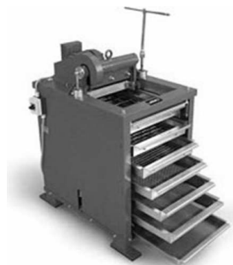
FIGURE 8: Series of sieves placed one above the other in order of size with the largest sieve at the top.
