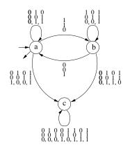
Figure 3: Automaton for the addition in base 2.
