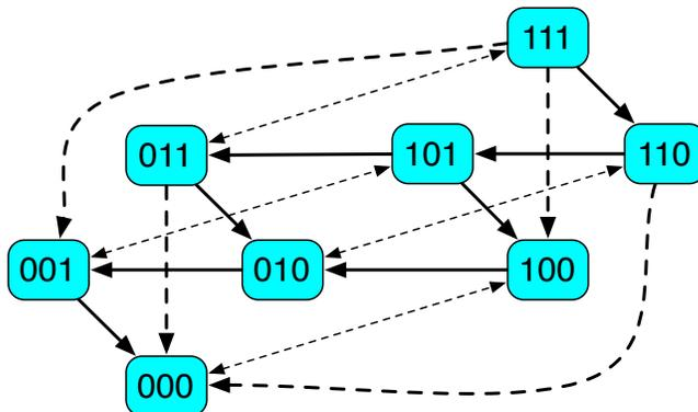
FIGURE 3. State transition diagram for  $n = 3$ . Solid arrows represent right shifts (including right annihilation), fat dashed arrows stand for annihilation in the bulk, thin dashed arrows indicate left creation and annihilation.
