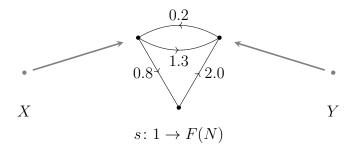
In the application to electrical circuits, the maps  $X \to N$  and  $Y \to N$  specify the inputs and outputs of the circuit, respectively, and are not required to be injective maps. In Section 5, we present an example where not all of the maps are injections. We can then compose these electrical circuits by identifying the inputs of one with the outputs of another. We refer the curious reader to Fong [9].
