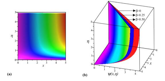
Figure 10: The flow streamlines in (a) two dimensions and (b) three dimensions when Maxwell parameter is varied.
