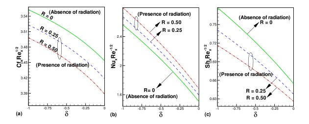
Figure 5: The effects of thermal radiation R and internal heat sink  $\delta$  on (a) reduced skin friction coefficient, (b) reduced Nusselt number and (c) reduced Sherwood number when  $\beta = \lambda = \tau = M = \gamma = N = Ec = 0.5$ , Pr = 5, Sc = 0.25 respectively.
