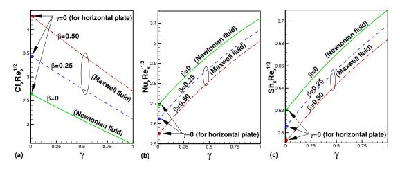
Figure 7: The effects of Maxwell parameter  $\beta$  and buoyancy parameter  $\gamma$  on (a) reduced skin friction coefficient, (b) reduced Nusselt number and (c) reduced Sherwood number when  $\beta = \lambda = \tau = M = N = R = Ec = 0.5$ , Pr = 5, Sc = 0.25,  $\delta = -1$  respectively.
