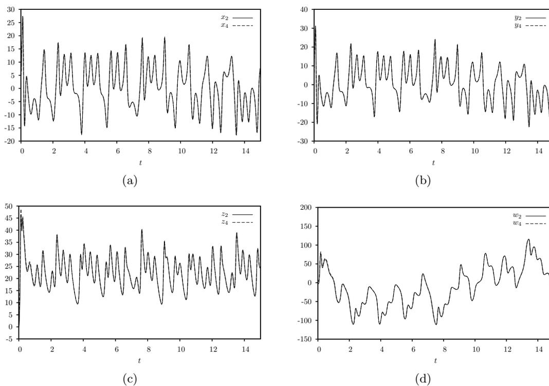
Figure 5: State trajectories between the pair of hyperchaotic Lü systems (4.2) and (4.4), (a) signals  $x_2$  and  $x_4$ ; (b) signals  $y_2$  and  $y_4$ ; (c) signals  $z_2$  and  $z_4$ ; (d) signals  $w_2$  and  $w_4$ .
