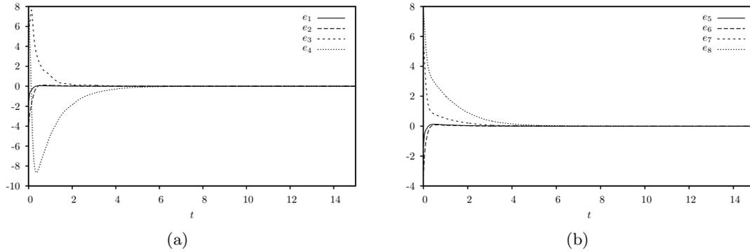
Figure 6: (a) The error signals  $e_1, e_2, e_3, e_4$  between the pair of hyperchaotic Chen systems; (b) The error signals  $e_5, e_6, e_7, e_8$  between the pair of hyperchaotic Lü systems.
