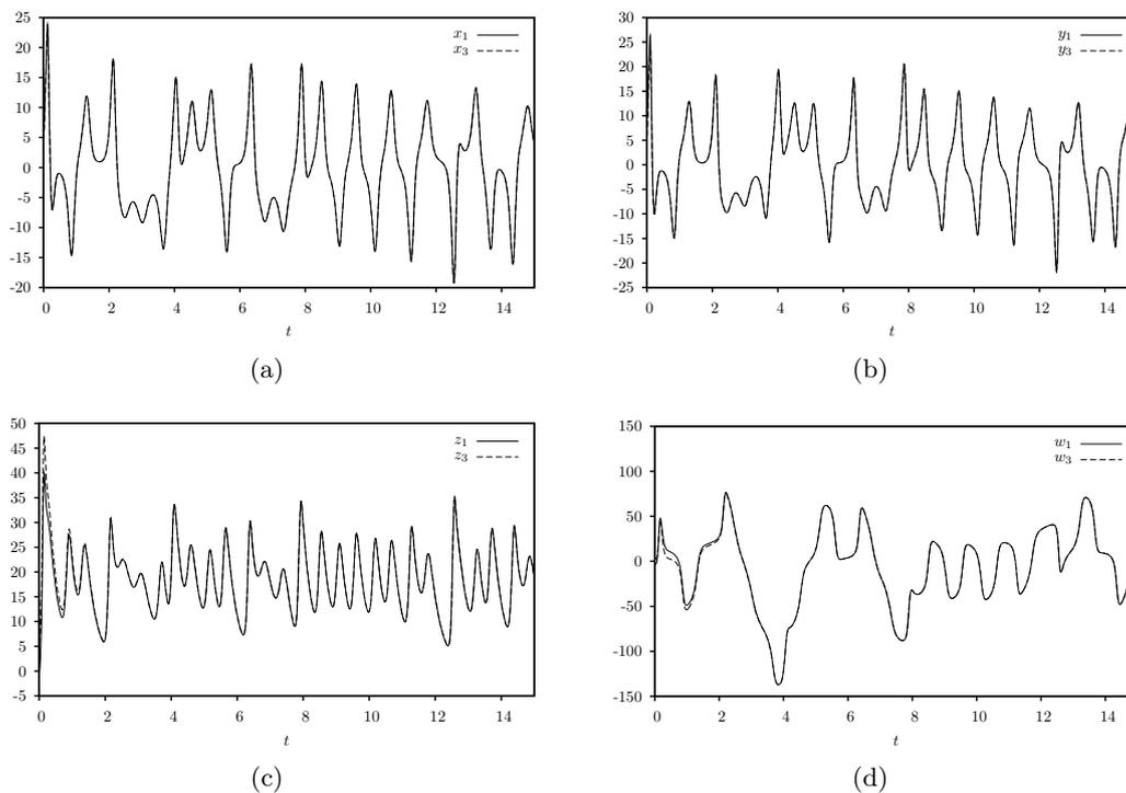
Figure 4: State trajectories between the pair of hyperchaotic Chen systems (4.1) and (4.3), (a) signals  $x_1$  and  $x_3$ ; (b) signals  $y_1$  and  $y_3$ ; (c) signals  $z_1$  and  $z_3$ ; (d) signals  $w_1$  and  $w_3$ .
