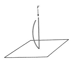
A rod bent under pressure. The bent position exhibits spontaneous symmetry breaking.
