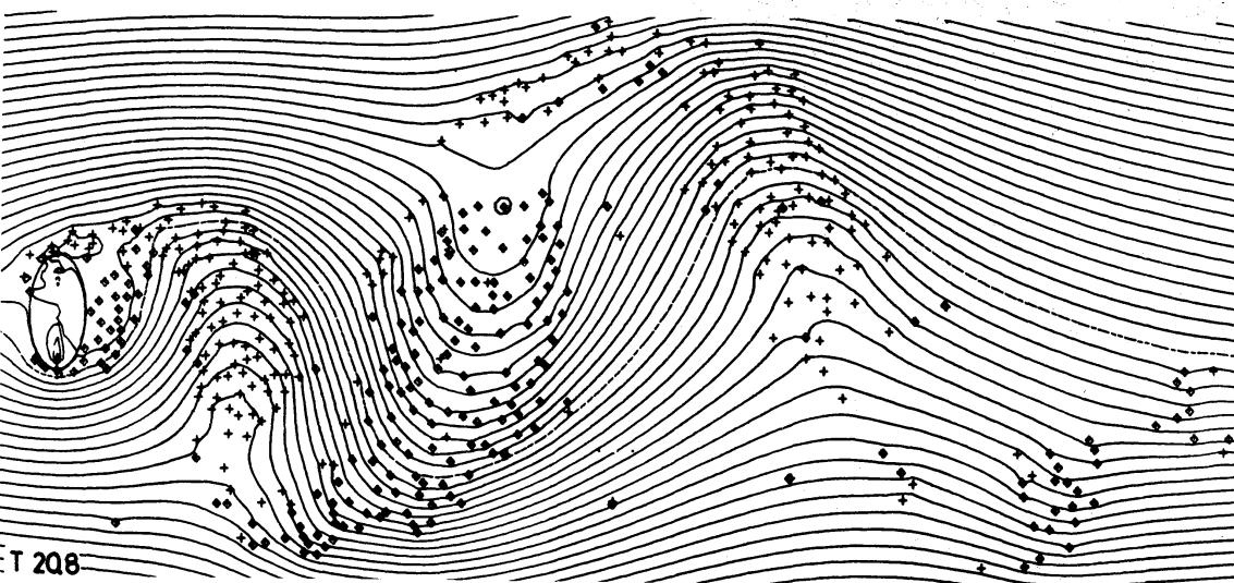
Fig.5 Vortex arrangements and stream lines (90°). Simpler case.
