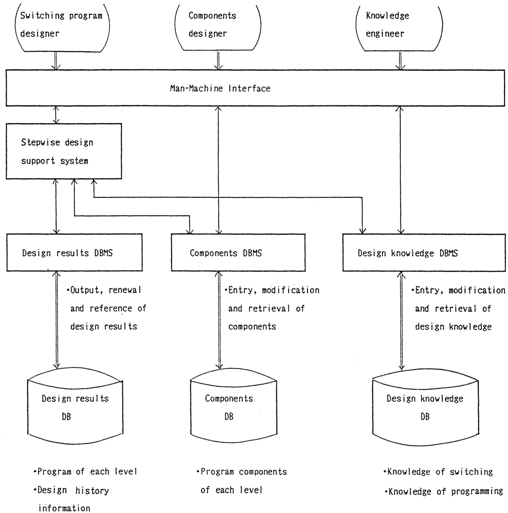
Fig. 3 Configuration of reusable design support system example
