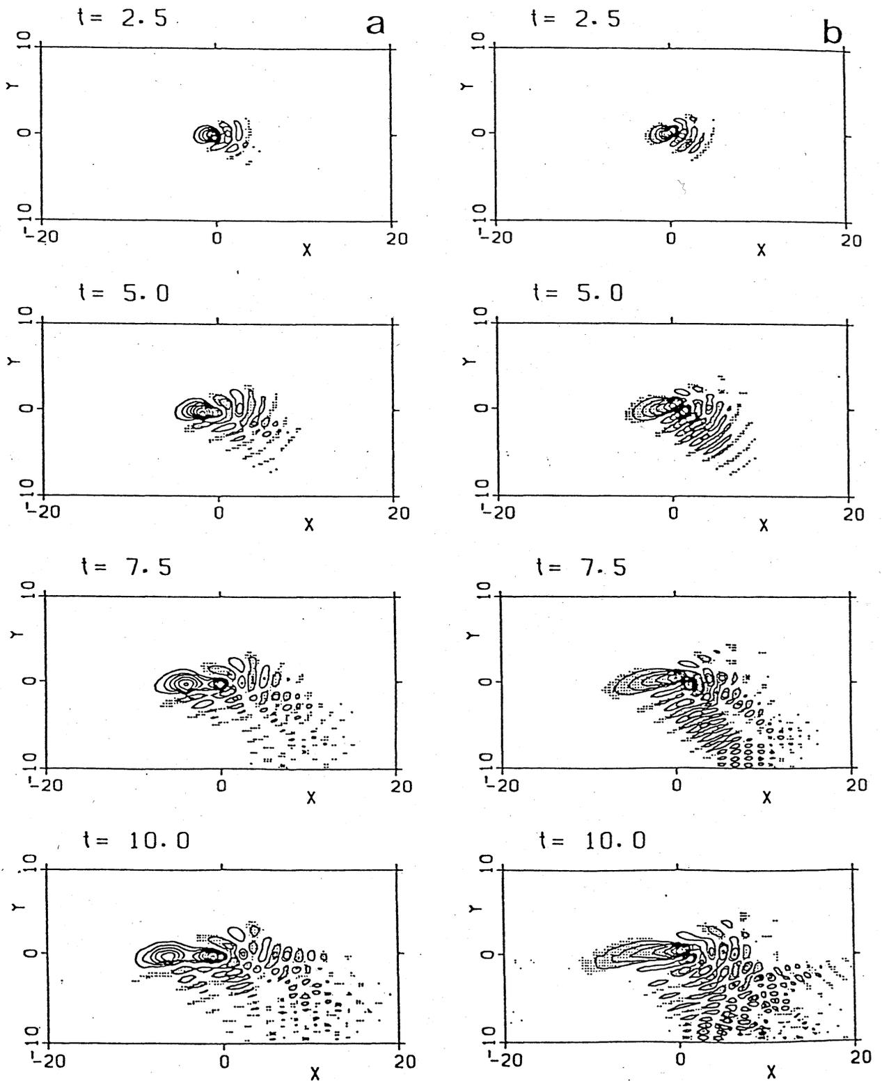
Figure 5. Evolution of the interface depression  $\eta$ . The forcing function is given by (3.5) in the text. (a) A case with positive forcing. (b) A case with negative forcing. The stippled areas represent negative values. The contour interval is 0.15.
