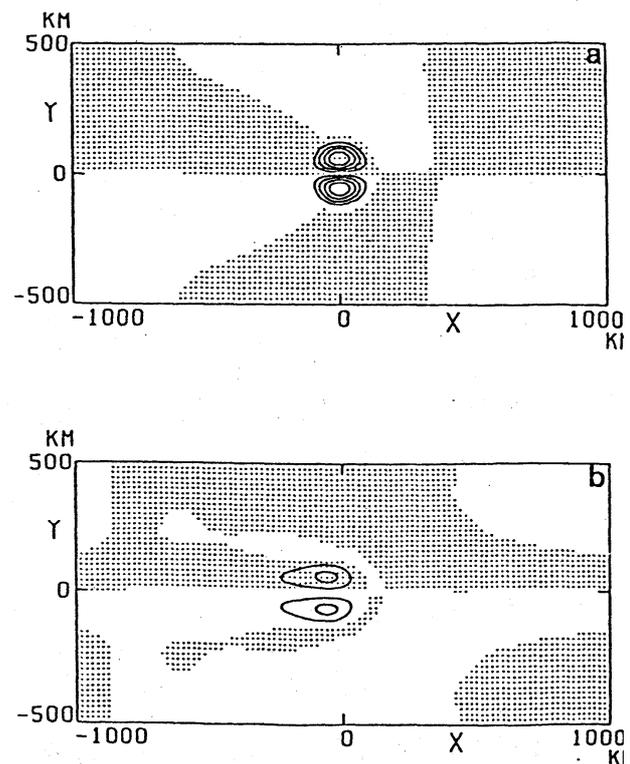
Figure 2. Streamfunction patterns for two distinct states for  $\lambda = 0.1 \times 10^{-1}$  /day. (a) High amplitude state of Stern's modon. (b) Low amplitude state of damped long Rossby waves. The stippled areas represent negative values. The contour interval is  $1.025 \times 10^7$  cm<sup>2</sup>/s, which corresponds to one fifth of the maximum value of  $\psi_b$ .
