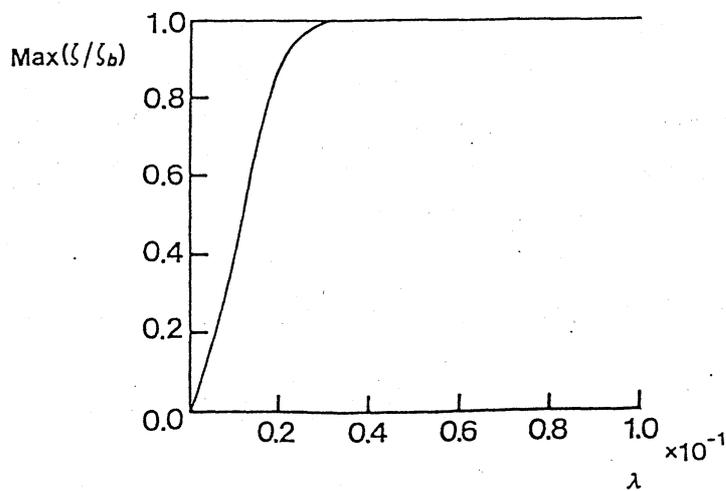
Figure 1. Normalized magnitude of maximum  $\zeta$  for the final steady state as a function of  $\lambda$ .
