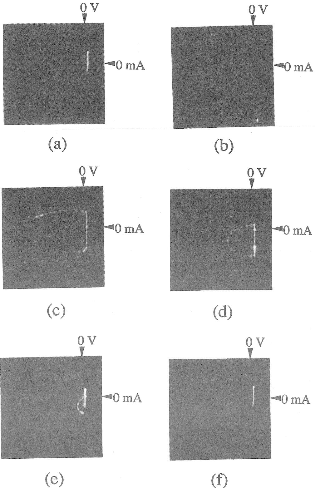
Figure 6 Observed cross sections of the *R-L-Diode* circuit at  $E=2.4$  V,  $f=50$  kHz. The horizontal axis is the diode voltage  $v_d$  (5.0 V/div) and the vertical axis is the inductor current  $i_L$  (2.0 mA/div). Since the origin is not located at the center of each figure, the axes are indicated by arrows.
