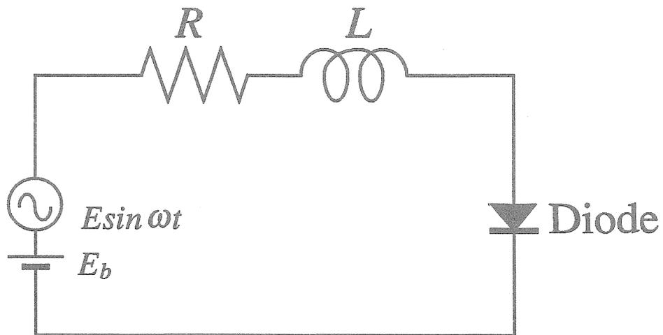
Figure 1 A driven  $R$ - $L$ - $\text{Diode}$  Circuit.
