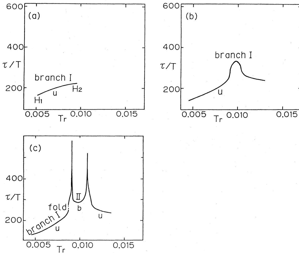
Fig.4  $T_r$ -dependence of periodic orbits. Solid and broken lines denote stable and unstable periodic orbits, respectively. u.p.o. and b.p.o. branches are expressed by  $u$  and  $b$ , respectively. (a)  $x_0/a = 0.001082$ , (b)  $0.001190$ , (c)  $0.001201$ .
