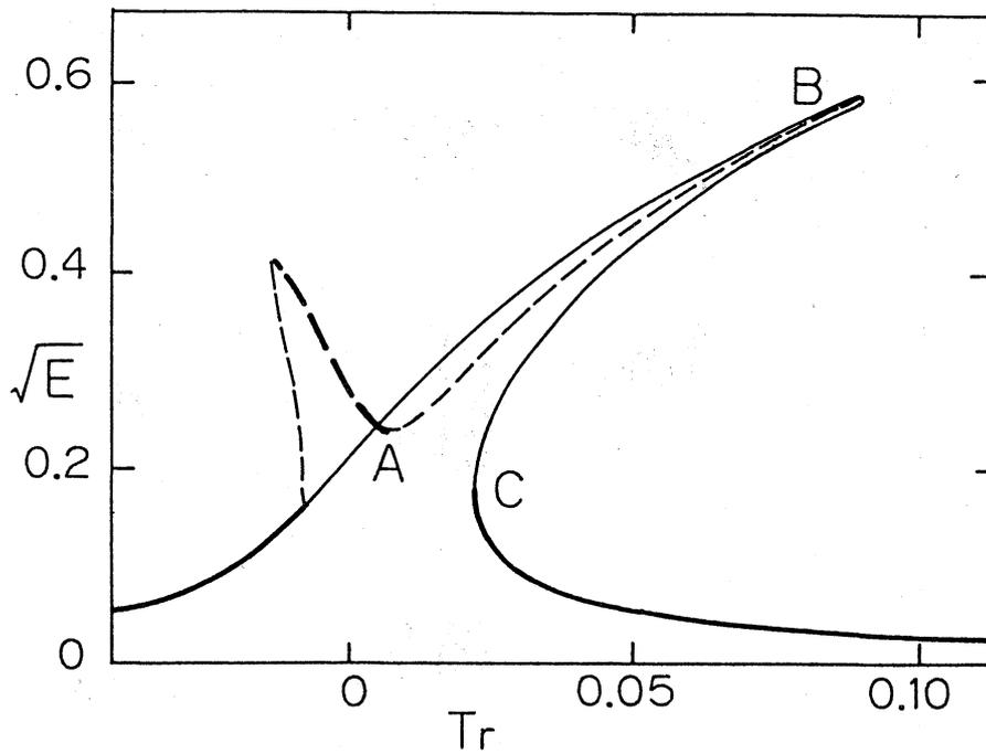
Fig.1 Typical  $T_r$ -dependence of fixed points. Solid line denotes the one-dimensional mode, and broken line the rotational mode. Bold and thin lines express stable and unstable fixed points, respectively.  $x_0=0.002706a$ .
