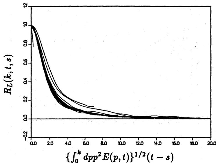
FIGURE 14. Time-scaled Lagrangian correlations for bands  $k = 2 + 5n$ ,  $n = 1 \dots 11$  for run SH.
