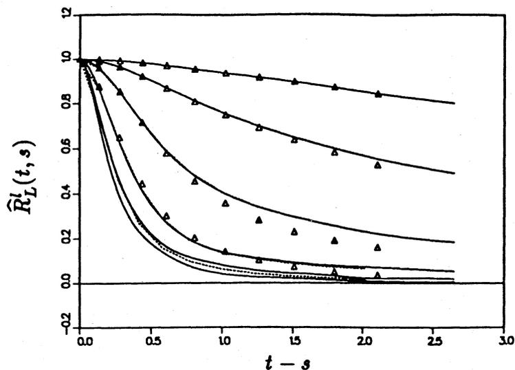
FIGURE 5. Lagrangian correlation within octave bands for run A. The uppermost curve corresponds to the lowest octave and the correlation decreases monotonically for successive octaves.
