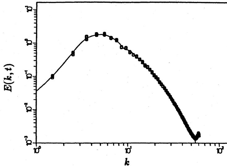
FIGURE 17. Energy spectrum for run SH. The spectra from the DNS are shown at 200 step intervals during the time span of  $R_L(t-s)$ .  $\circ$  DNS, and — the spectrum used in the MLRA (time averaged DNS energy spectrum).
