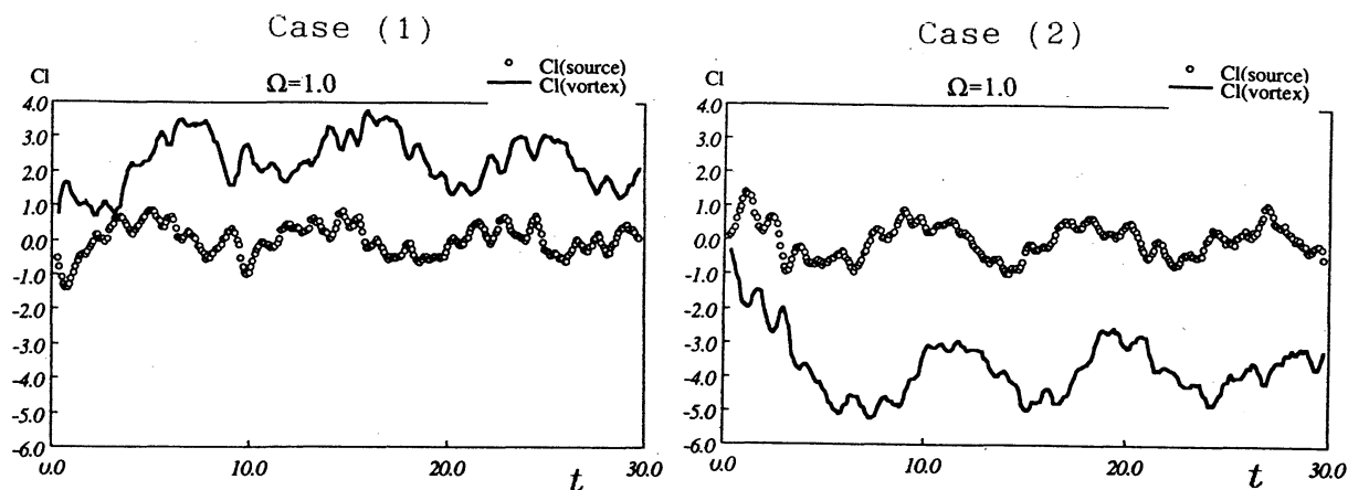
Fig.9. Lift components of shedding vortex and others
