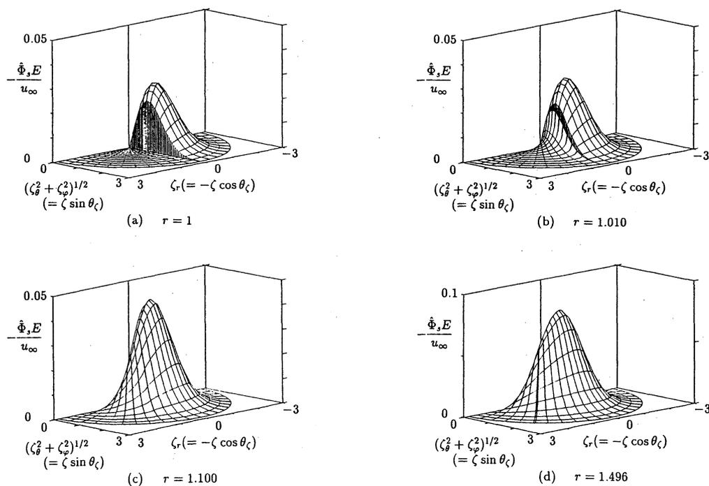
FIG. 7. The velocity distribution function  $\hat{\Phi}_s E$  at four points in the gas for  $k_\infty = 0.1$ . (a)  $r = 1$ , (b)  $r = 1.010$ , (c)  $r = 1.100$ , and (d)  $r = 1.496$ . The surface of  $\hat{\Phi}_s E$  is shown as a function of  $\zeta \cos \theta_\zeta$  and  $\zeta \sin \theta_\zeta$  by lines  $\zeta = \text{const}$  and  $\theta_\zeta = \text{const}$ . The vertical stripes show the discontinuity. Note the difference of the ordinate in Fig. 7d.
