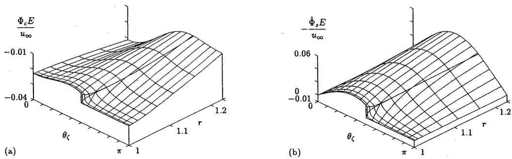
FIG. 14. The velocity distribution functions  $\Phi_c E$  and  $\hat{\Phi}_s E$  at  $\zeta = 0.556$  for  $k_\infty = 0.1$ . (a)  $\Phi_c E$  and (b)  $\hat{\Phi}_s E$ . The surfaces of  $\Phi_c E$  and  $\hat{\Phi}_s E$  are shown as functions of  $r$  and  $\theta_\zeta$  by lines  $r = \text{const}$  and  $\theta_\zeta = \text{const}$ . The vertical lines show the discontinuity. The invisible lines behind other parts are shown by dashed lines.
