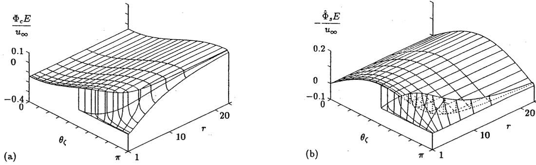
FIG. 16. The velocity distribution functions  $\Phi_c E$  and  $\hat{\Phi}_s E$  at  $\zeta = 0.556$  for  $k_\infty = 10$ . (a)  $\Phi_c E$  and (b)  $\hat{\Phi}_s E$ . (See the caption of Fig. 14.)
