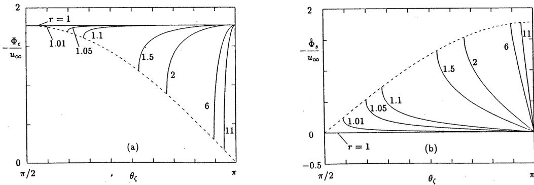
FIG. 13. The velocity distribution functions  $\Phi_c$  and  $\hat{\Phi}_s$ , for  $\pi - \text{Arcsin}(1/r) < \theta_\zeta \leq \pi$  (the molecules coming directly from the sphere) in the free molecular flow [Eqs. (23) and (24)]. (a)  $\Phi_c$  and (b)  $\hat{\Phi}_s$ .
