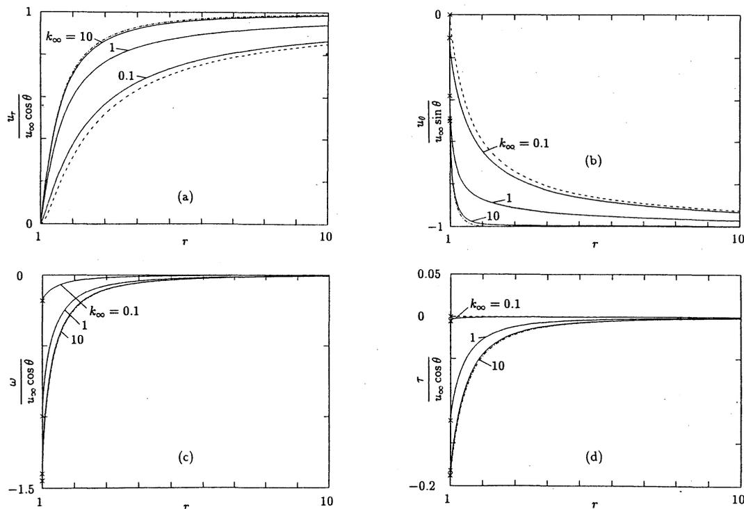
FIG. 3. The profiles of the macroscopic variables (hard sphere). (a)  $u_r/u_\infty \cos \theta$  vs  $r$ , (b)  $u_\theta/u_\infty \sin \theta$  vs  $r$ , (c)  $\omega/u_\infty \cos \theta$  vs  $r$ , and (d)  $\tau/u_\infty \cos \theta$  vs  $r$ . Here, — indicates the present numerical result, - - - the asymptotic solution (26a)-(26d) with  $k_\infty = 0$ , and ···· the free molecular flow ( $k_\infty = \infty$ ). The  $\times$  indicates the value at  $r = 1$ .
