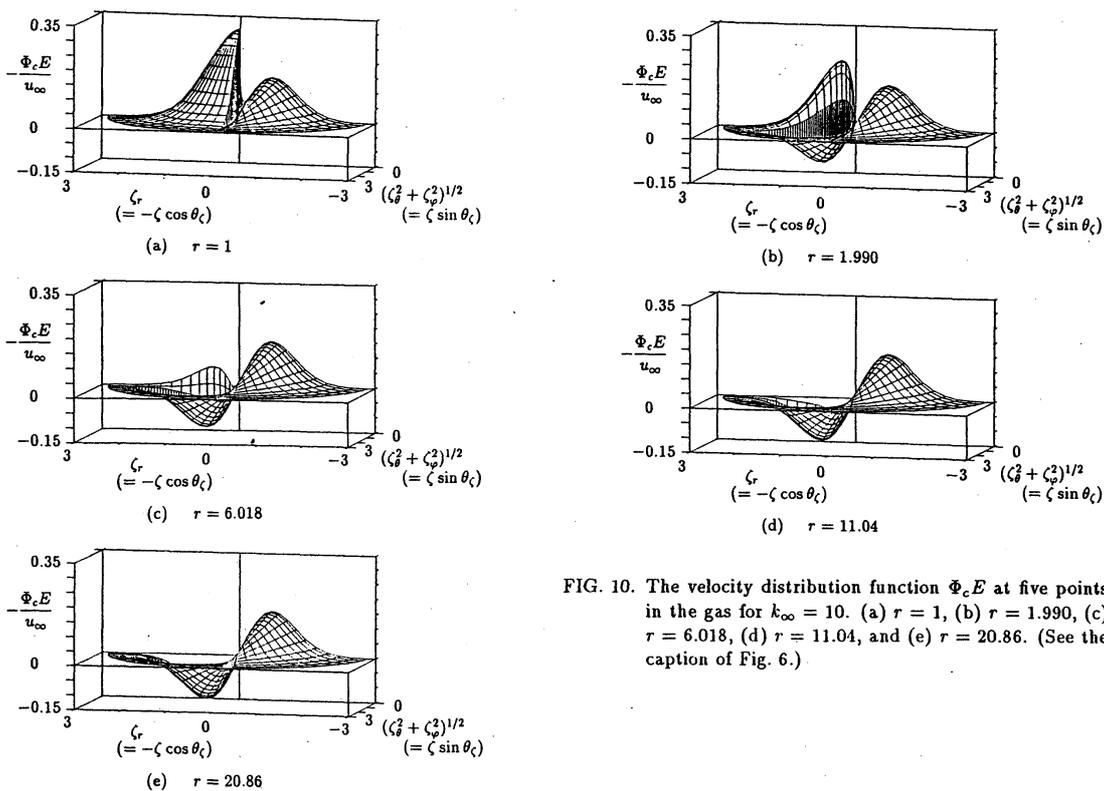
FIG. 10. The velocity distribution function  $\Phi_c E$  at five points in the gas for  $k_\infty = 10$ . (a)  $r = 1$ , (b)  $r = 1.990$ , (c)  $r = 6.018$ , (d)  $r = 11.04$ , and (e)  $r = 20.86$ . (See the caption of Fig. 6.)
