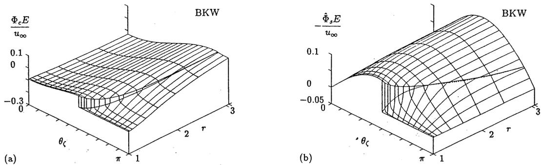
FIG. 18. The distribution functions  $\Phi_c E$  and  $\hat{\Phi}_s E$  for the BKW equation at  $\zeta = 0.667$  for  $k_\infty = 1$ , which corresponds to Fig. 15 (hard sphere). (a)  $\Phi_c E$  and (b)  $\hat{\Phi}_s E$ . (See the caption of Fig. 14.) The conversion (58) of  $k_\infty$  is not made here. Note the difference of the value  $\zeta$  from that in Fig. 15.
