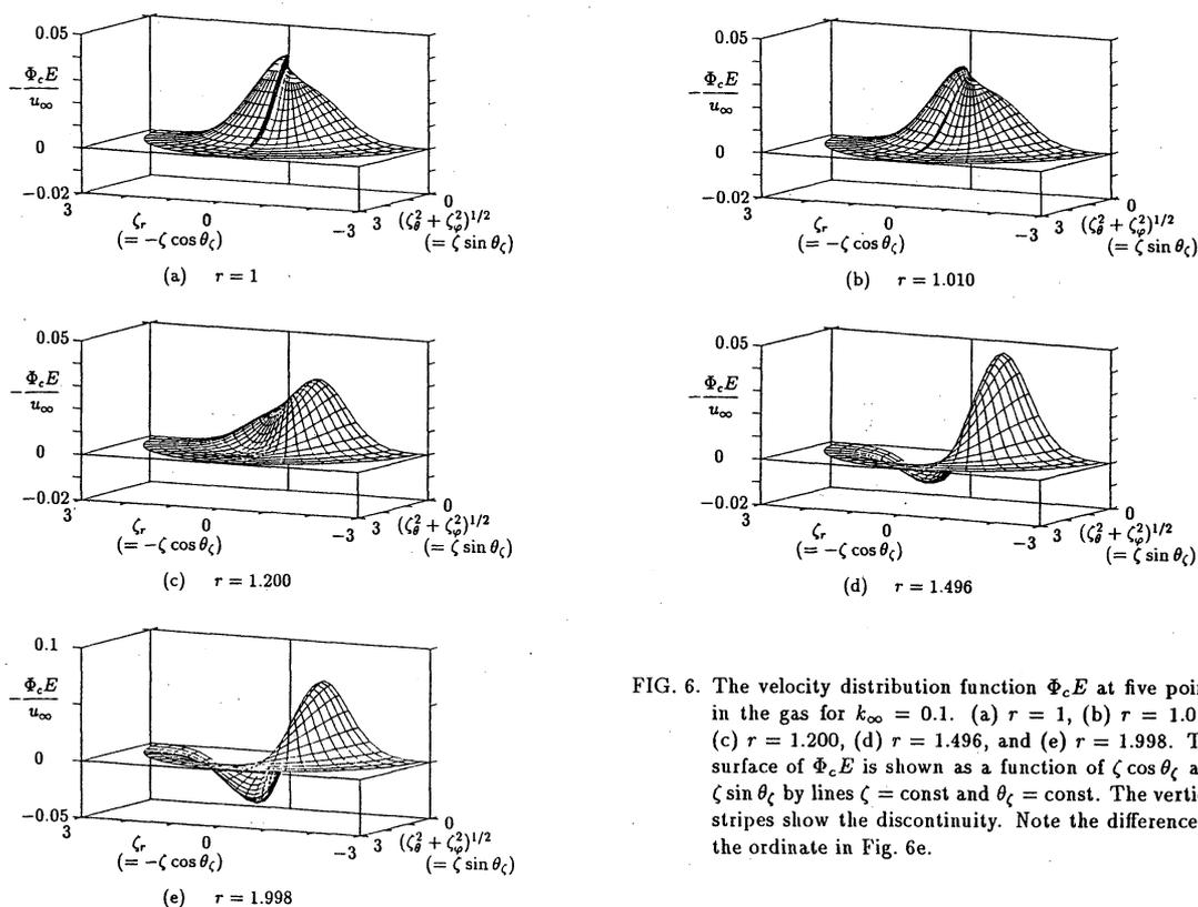
FIG. 6. The velocity distribution function  $\Phi_c E$  at five points in the gas for  $k_\infty = 0.1$ . (a)  $r = 1$ , (b)  $r = 1.010$ , (c)  $r = 1.200$ , (d)  $r = 1.496$ , and (e)  $r = 1.998$ . The surface of  $\Phi_c E$  is shown as a function of  $\zeta \cos \theta_\zeta$  and  $\zeta \sin \theta_\zeta$  by lines  $\zeta = \text{const}$  and  $\theta_\zeta = \text{const}$ . The vertical stripes show the discontinuity. Note the difference of the ordinate in Fig. 6e.
