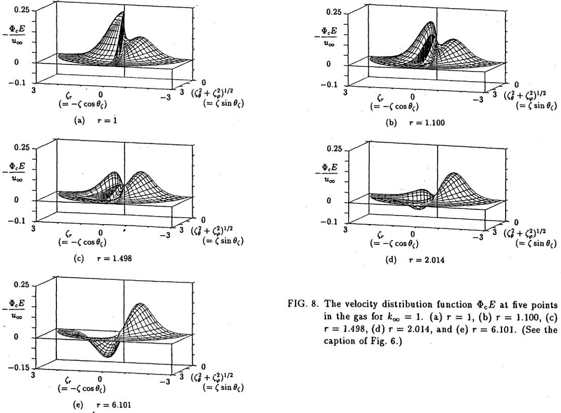
FIG. 8. The velocity distribution function  $\Phi_c E$  at five points in the gas for  $k_\infty = 1$ . (a)  $r = 1$ , (b)  $r = 1.100$ , (c)  $r = 1.498$ , (d)  $r = 2.014$ , and (e)  $r = 6.101$ . (See the caption of Fig. 6.)
