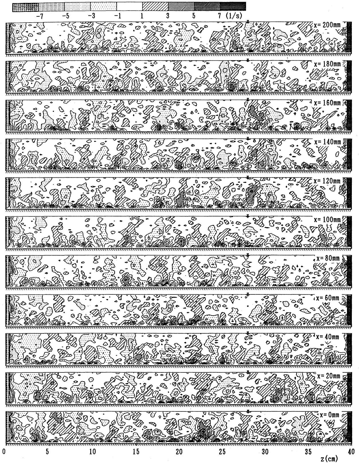
Fig.6 The contours of the vertical component of vorticity in transverse cross-sections.
