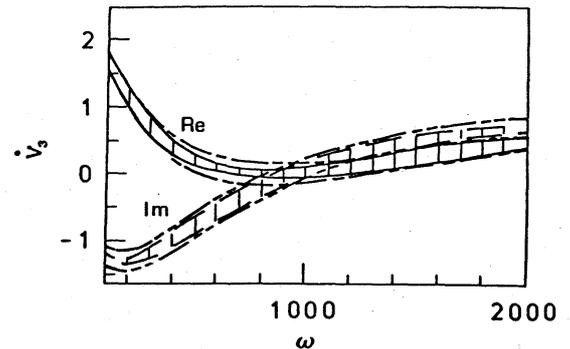
Fig. 2 The frequency characteristics of the voltage  $V_3$ .
