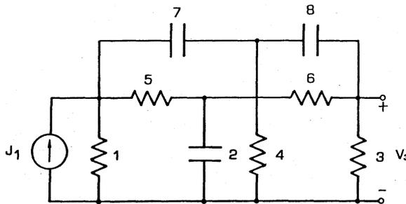
Fig. 1 Notch filter circuit.
