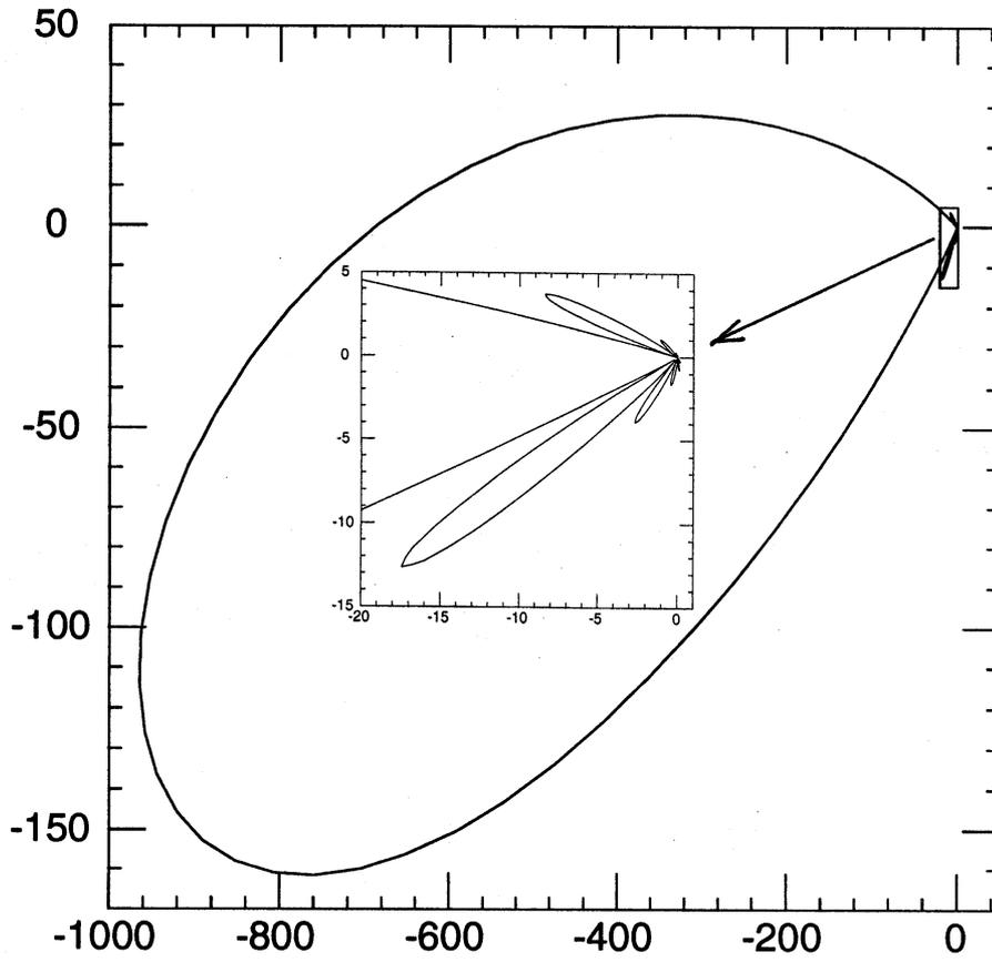
Figure 3. Polar plot of differential cross section for  $\alpha = 1$  and  $\beta = 10$ . The incident wave comes from the right side.
