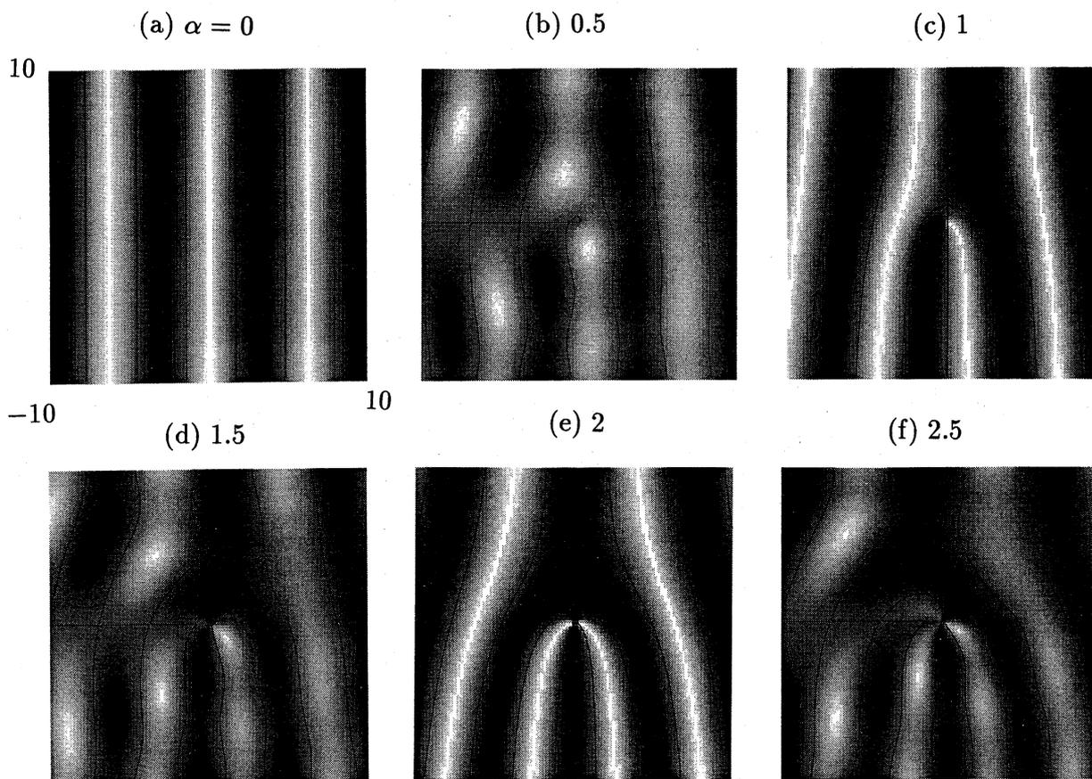
Figure 1. Density plots of incident dislocated waves for  $\alpha =$  (a) 0, (b) 0.5, (c) 1, (d) 1.5, (e) 2 and (f) 2.5 The summation in (48) is truncated at  $n = \pm 20$ . The plotted region is  $-10 \leq x \leq 10$  and  $-10 \leq y \leq 10$ . Lines denote the zero displacement.
