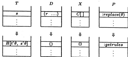
In the meta-replace step, the current subject term will become  $H[t'\theta, z'\theta]$ , and the stacks  $D$  and  $X$  are initialized.  $H$  is the primitive function symbol of arity 2.
