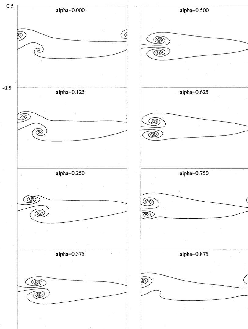
Figure 13: The numerical solutions of two sheet with the various initial phase differences  $\alpha = 0.0, 0.125, 0.25, 0.375, 0.5, 0.625, 0.75, 0.875$ . The initial difference between them are fixed to  $H = 0.2$ .
