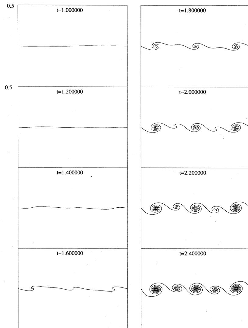
Figure 4: Time evolution of the vortex sheet.  $G = 1.5\pi$ . Singularities grow in number from one to five.
