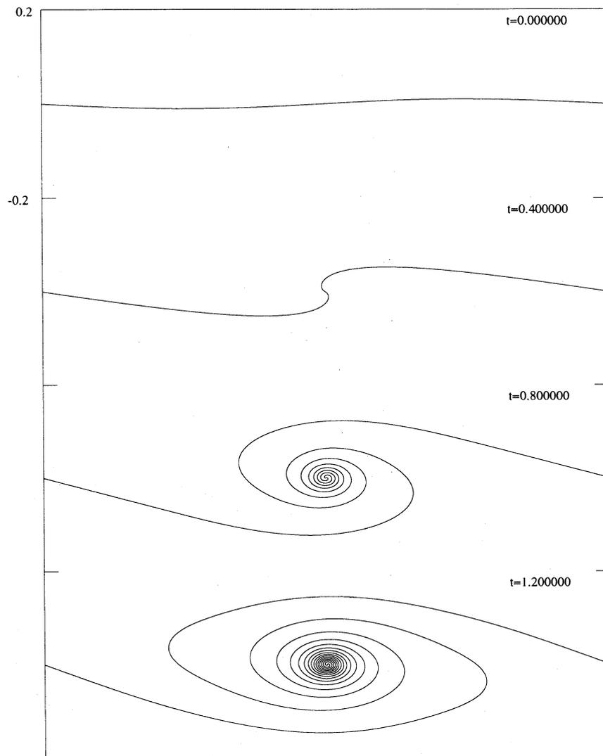
Figure 2: Time evolution of the vortex sheet.  $G = -1.5\pi$ . Qualitatively the same as Figure 1 but the roll-up appears earlier and the roll size is more oblate.
