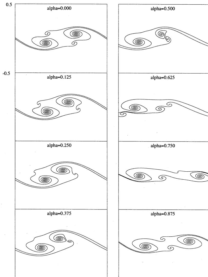
Figure 10: The numerical evolution of two vortex sheet in condition with various  $\alpha$  at time  $t = 1.0$ . The initial phase difference is fixed to  $H = 0.1$ .
