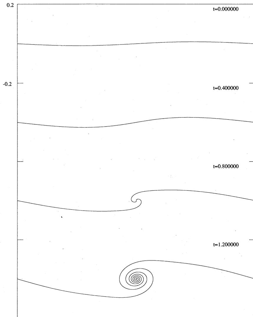
Figure 3: Time evolution of the vortex sheet.  $G = 0.5\pi$ .
