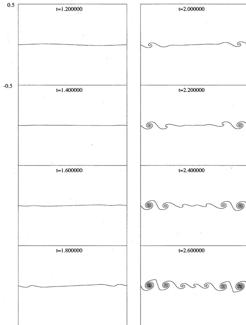
Figure 5: Time evolution of the vortex sheet.  $G = 2.5\pi$ .
