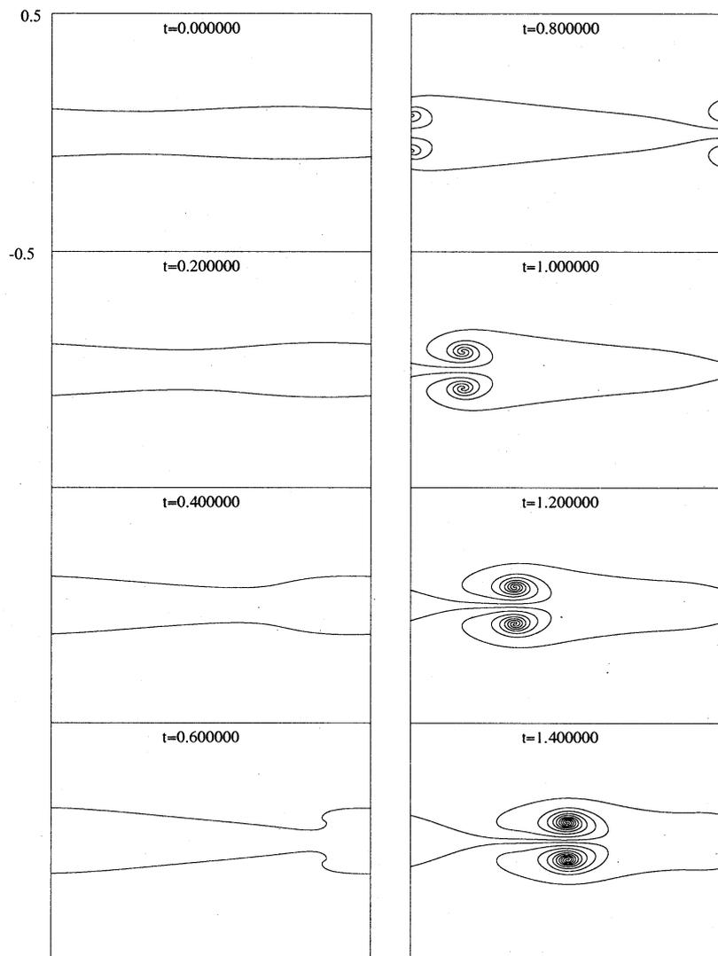
Figure 11: The evolution of two vortex sheets. Initial conditions of two vortex sheets are  $\sigma_1 = 1, \sigma_2 = -1, H = 0.2$ , and  $\alpha = 0.5$  (symmetric with respect to x-axis).
